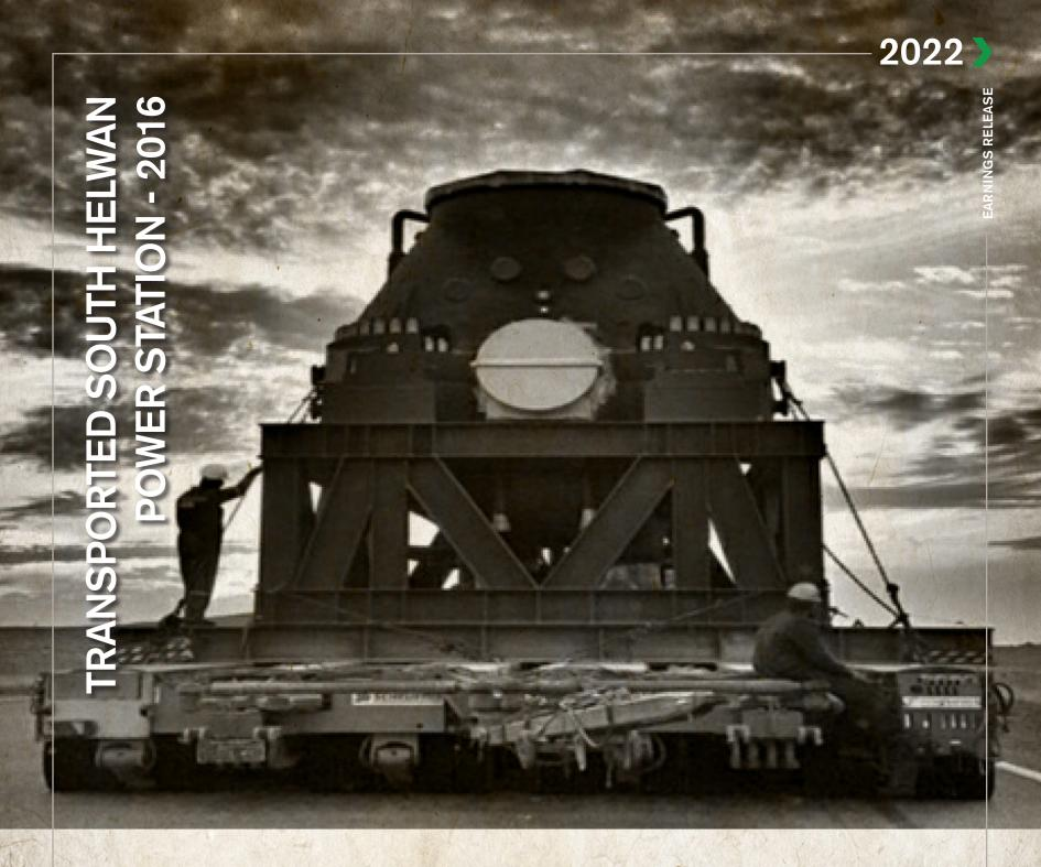
Egytrans transported and discharged 255 tons turbine for South Helwan Power Station. The Turbine is 9.10 m long, 4.90 m wide and 5.40 m high.
